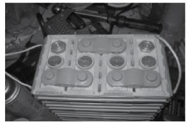
Nominal Pack voltage 72V (6 batteries in series) Config (two parallel strings of 6 batteries each, for 12 batteries total) The 6 batteries in series are tied together at the controller. Chargers – 4 Dual Pro 3 chargers (each charger has 3 leads to
